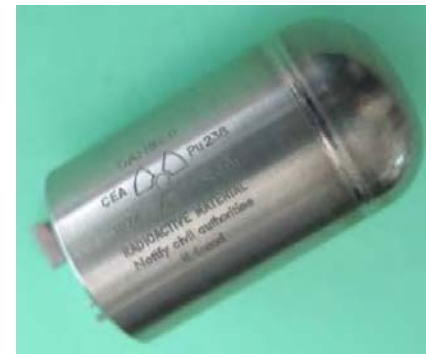
Miniature plutonium power for pacemaker
